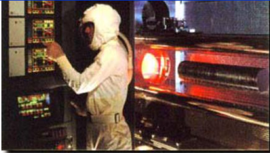
Oxidation Furnace (Silicon Valley Group - Thermco Systems)
